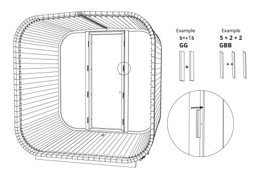
**STEP 20**: Fix one side of the door cabinet with screws(**S14**)slightly outwards over the spacers. Then insert the spacers on the other side. Connect the spacers to the required width. The spacers must
