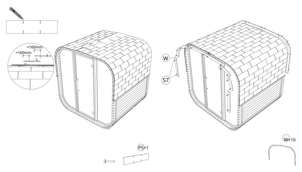
**STEP 38**: Use bitumen sealant behind the decorative boards to fill the gap between the shingle and the boards.
