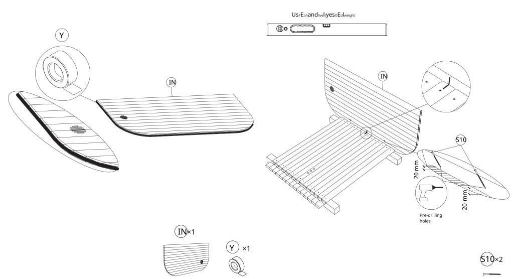
**STEP 6**: Along the edges of both front panels**(F)**Apply adhesive tape. Insert a wooden dowel into both holes at the top and bottom of the front panel. Pre-drill holes in the panel sill, evenly spaced and not too close to the sides.
