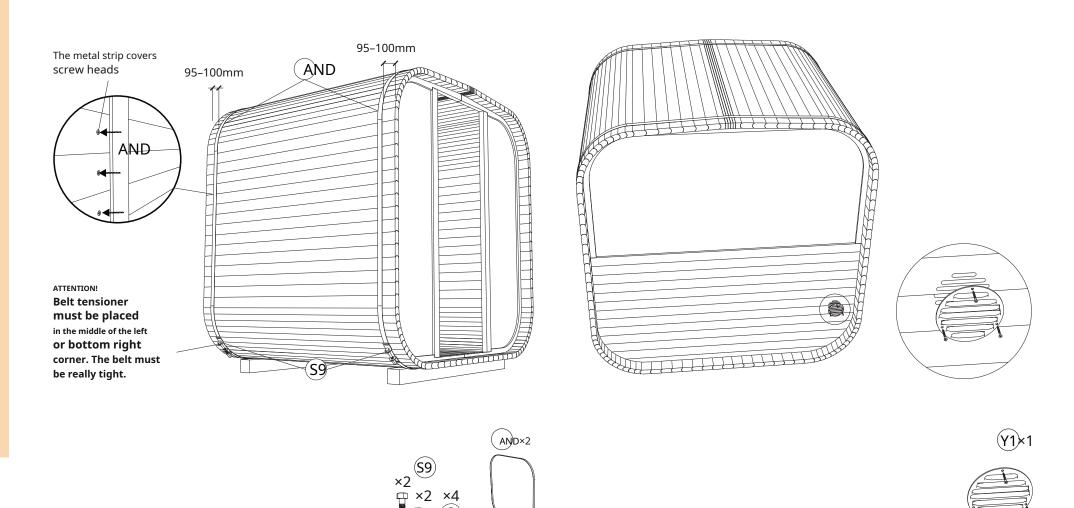
**STEP 18**: Install the door(**F2**). Place the door on the threshold and place it in the frame approximately in the middle. Secure the door with clamps or have another person hold it.
