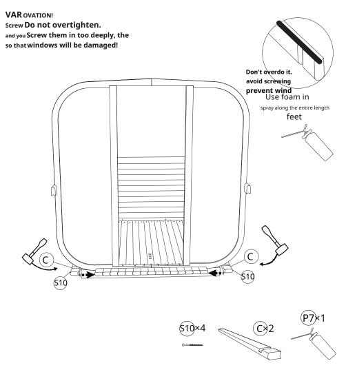
**STEP 10**: Attach 12 feet(**SC**)on both s For a firmer fit, use rubber mallets. When both corners are finished, remove the connecting
