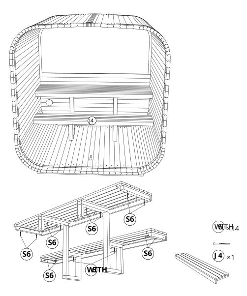
STEP 25: Install the bench legs( installJ1)using screws(S6)The left foot is needed next to the front panel(F panel. Attach), the right leg is 750 mm from the lower rear the sauna bench(J8) using screws(S6).
