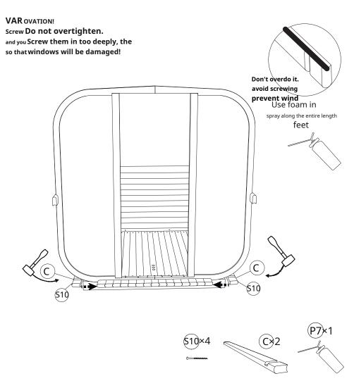
**STEP 10**: Attach 12 feet(**SC**)on both s For a firmer fit, use rubber mallets. When both corners are finished, remove the connecting
