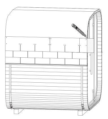
**STEP 34**: Continue laying shingles until the last layer passes over the center of the roof.
