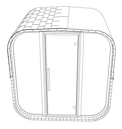
STEP 35: Repeat the same process Use a heat source until the last layer is tacky. Lift each across the center of the roof. For better rectangle, adhesion, heat it a little and press it to E roof.
