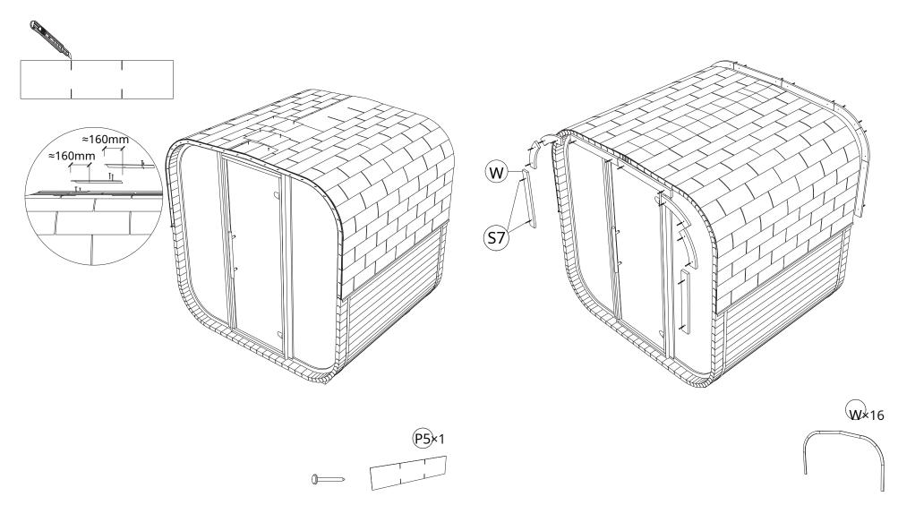
**STEP 38**: Use bitumen sealant behind the decorative boards to fill the gap between the shingle and the boards.
