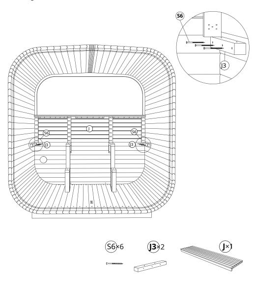
**STEP 24**: Using(**S6**)install the bench(**J**)on the top of the legs(**J6**). The bench cross-boards must match the tops of the bench legs. Attach the bench step(**J4**) using screws(**S6**).
