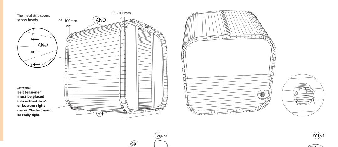
**STEP 18**: Install the door(**F2**). Place the door on the threshold and place it in the frame approximately in the middle. Secure the door with clamps or have another person hold it.
