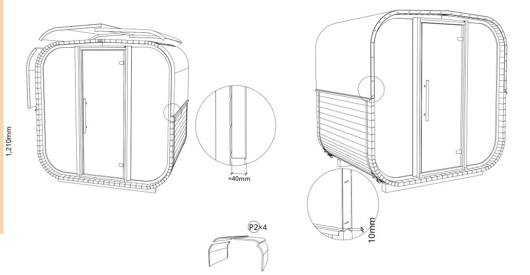
**STEP 30**: Remove the protective film next from the bottom of the sheet. Place the beginnings nshingles to each other. Then attach them with nails to shown in the picture. Cut off before nailing. neat to the excess part of the startershingle.
