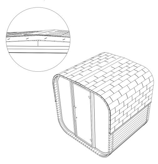
**STEP 36**: Use starter shingles for the top of the roof. Cut several shingles into squares, with lines marked on them. Remove the protective film. Nail each shingle with two nails. The next shingle goes about 160 mm from the previous one. When finished, use a heat source for better adhesion.
